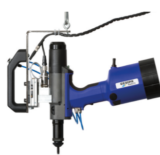
FireFox® 2 F Axial eco with contact pressure monitoring and counting sensor
