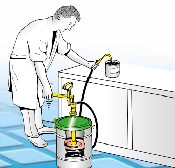
Transfer in small drums
