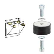
P/N KR33/88 Antivibration kit in SBR rubber ø 30 x h. 20 thread F/F - M12 for 1.1/2" and 2" diaphragm pump. It reduces the vibrations in heavy applications.
